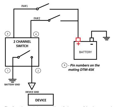
**Note**: The inputs each have a 1k pull down resistor to ground.
