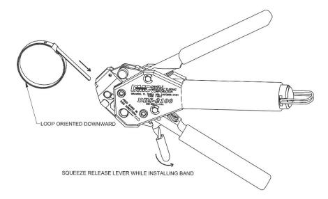
Step 4: Tighten Band around Braid/Connector
