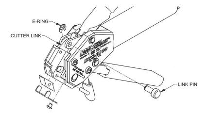
• Rotate Cutter Link so that the dowel pin becomes visible in the large access hole.
