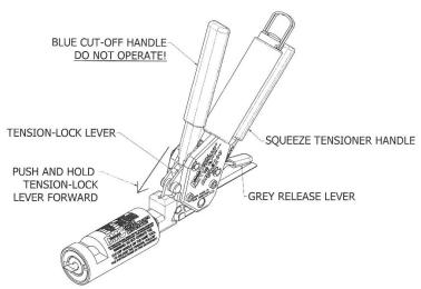
NOTE: <u>DO NOT ATTEMPT TO CUT THE BAND</u>. DAMAGE TO THE TOOL AND/OR GAGE MAY OCCUR.
