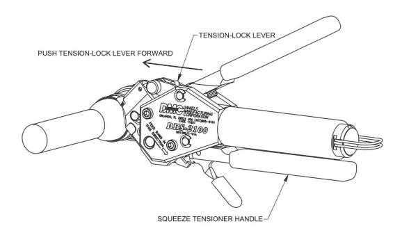
To loosen or remove the looped band after locking the tensioner handle at the precalibrated tension, squeeze the tensioner handle and push the tension-lock lever forward. While holding the tension-lock lever forward, release the tensioner handle. The tensioner handle will open fully. Squeeze the release lever and pull the looped band away from the nose of the tool.
