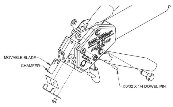
To replace blades, reassemble in reverse order. Assemble the #4-40 button head screw with Loctite 242 or equivalent to prevent the screw from backing out during use.
