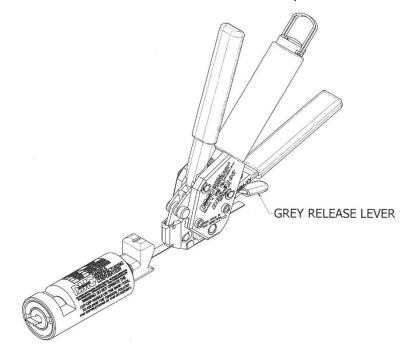
Step 3: Align the tool with the verification inspection gage
