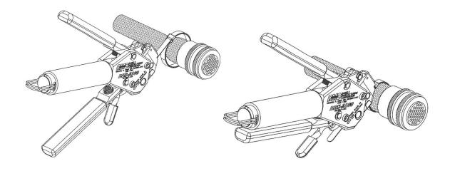
Apply an adequate amount of pressure in line with the cable as it enters the backshell to allow the 1/8 inch space to be reduced to zero. The tool is then activated to the preset tension, and terminated/cut using the procedure described in section 1.0 of this guide.
