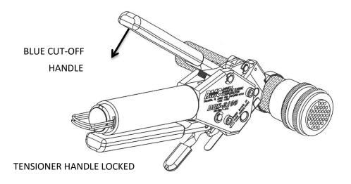
**Step 6: Remove excess band material**
