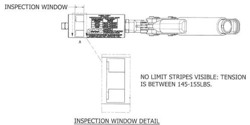
If any amount of the yellow stripe is visible, the tension applied to the band by the DBS-2100 is above 155LBS. This indicates that the tension setting for the DBS-2100 must be adjusted. (See section 3.2 for adjustment instructions.)
