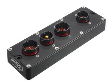
MoTeC's 32 output Power Distribution Module is designed to provide electronically switched power to the various electrical systems in the vehicle such as motors, lights, solenoids, and electronic devices such as ECUs and data acquisition systems.
