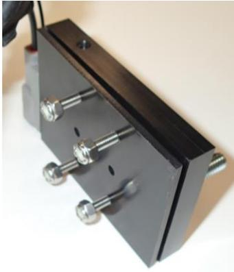
Remove the nut, washers, lugs and relay to access the mounting screws. Use the provided 8-32 screws. Once secured, return the washers, lugs and relay in the order shown below. The provided mounting plate must be used behind the relay block to prevent accidental shorting of the power studs to the mounting location.
